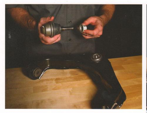
a strut assembly that incorporates a combined coil spring/strut assembly. The ball joints attach to the ends of the control arms. Control arms themselves rarely wear out, but related bushings or the ball joints may need servicing, sometimes involving the whole control arm assembly.
